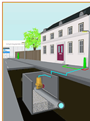
TrunkMinder, a permanent on-line leak monitoring system for trunk mains.
